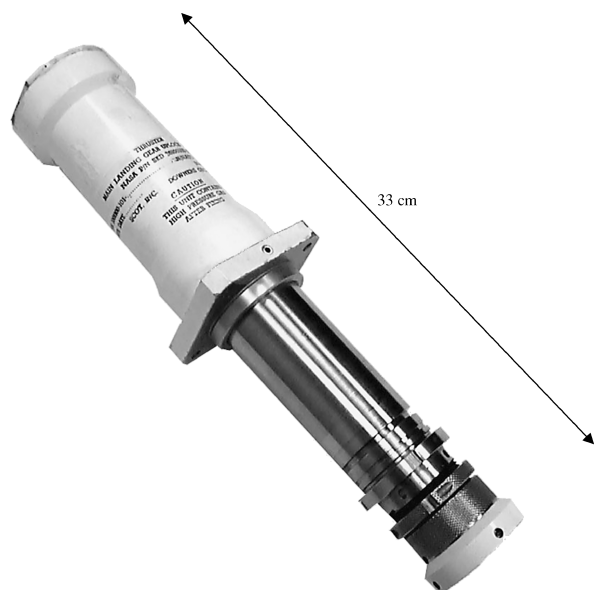
Fig. 1a Photograph of pyrotechnic thruster used for an emergency landing scenario for the space shuttle.
